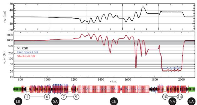
Figure 2: The bunch compression scheme for the Cornell ERL in the high energy user region.
