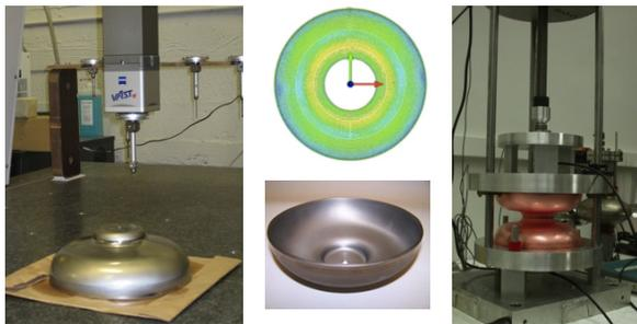
Figure 7: Verification of cell shape. Left: Coordinate measurement machine (CMM) scanning of half cells. Middle: CMM results show that cell shape errors are within 0.125 mm after deep drawing. Right: Frequency check of finished dumbbells used to determine equator trim dimensions for correct frequency.
