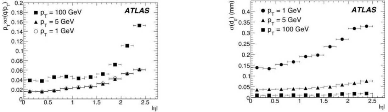
FIG. 4:  $p_T$  (left) and impact parameter (right) resolutions for ATLAS Inner tracker
