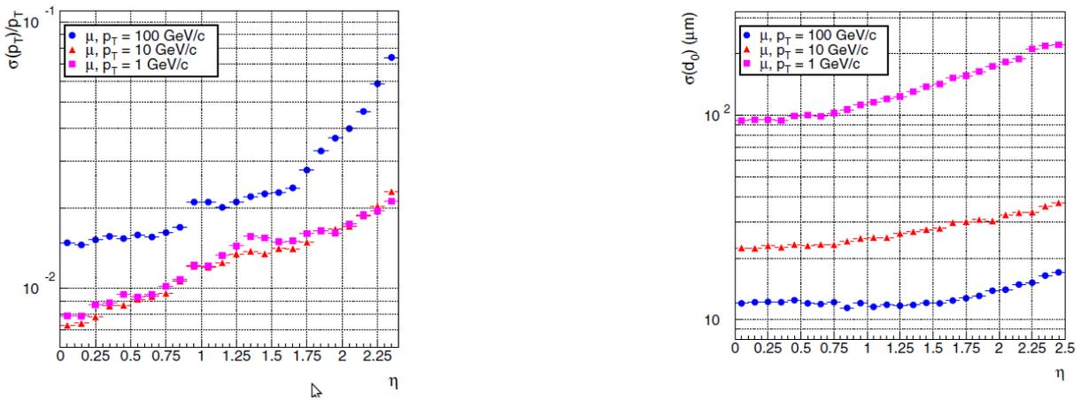
FIG. 5:  $p_T$  (left) and impact parameter (right) resolutions for CMS Tracker (Pixel and Silicon Strip combined)
