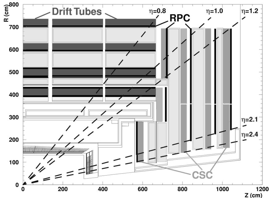
FIG. 6: CMS Muon system
