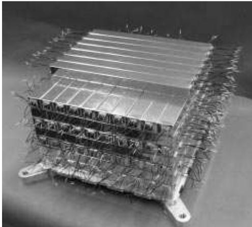
FIG. 2: Hodoscopic lay out of the CsI crystals in the LAT
