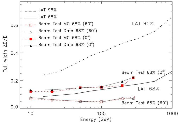
FIG. 3: Energy Resolution for electrons up to 1 TeV
