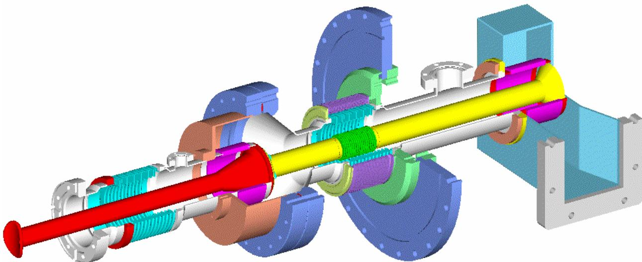
Figure 3: View of the injector cavity coupler.
