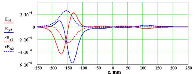
Figure 4: Normalized transverse fields on the axis of the injector cavity for a relative penetration depth error of 1 mm. The coordinate  $z = 0$  corresponds to the cavity center.  $E_{y1}$ ,  $B_{x1}$  and  $E_{y2}$ ,  $B_{x2}$  were calculated respectively for shorted and open coupler.
