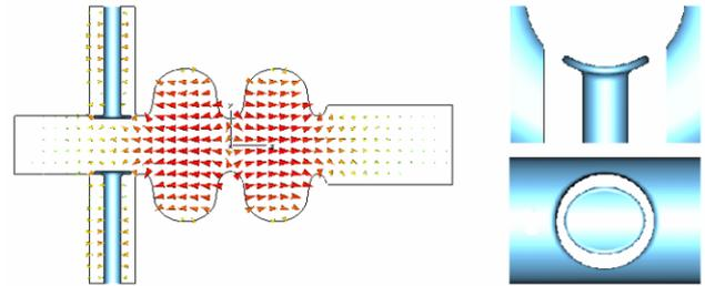
Fig. 1. Geometry of the cavity with the fundamental mode excited in it and details of the coupler.
