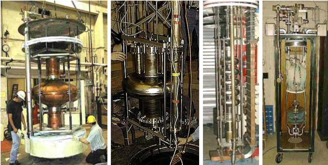
Figure 6: Cavity test inserts for various frequencies. From left to right: 200 MHz system, 500 MHz system, 1300 MHz system and 1500 MHz system.
