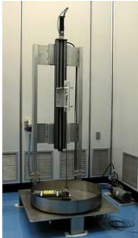
Figure 3: New high-pressure water rinsing system.
