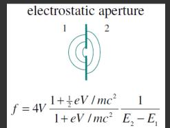
E.g.  $V = 500 \ kV$ , gap = 5cm $\Rightarrow f_{anode} \sim -15 \ cm$
