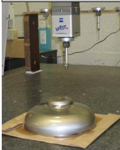
Quality control: CMM and frequency check
