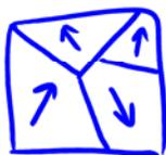
Domains can get pinned on crystal defects,  $\Rightarrow$  hard (permanent) magn.
