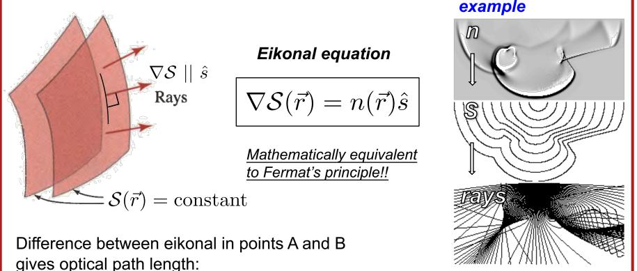
$$\mathcal{S}(\vec{r}_B) - \mathcal{S}(\vec{r}_A) = \int_A^B |\nabla \mathcal{S}| \, ds = \int_A^B n \, ds = \text{optical path length}$$
