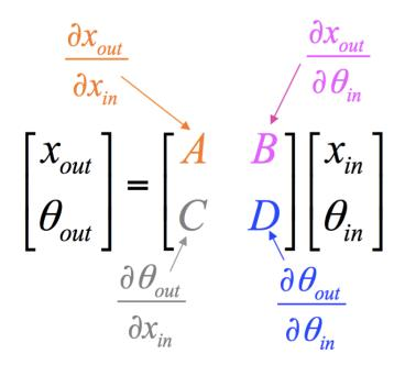
$X_{out}$  $= \frac{\partial \theta_{out}}{\partial x_i} x_{in} + \frac{\partial \theta_{out}}{\partial \theta_i} \theta_{in}$  $\theta_{out}$
