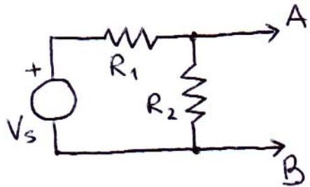
Useful trick: to find  $R_{Th}$ , short \_\_\_\_\_ and open \_\_\_\_\_.  $R_{Th}$  is resistance by looking inside the two terminals.
