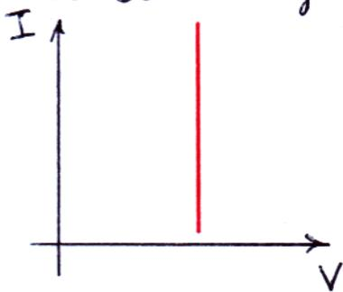
slope =  $\infty = \frac{1}{R} \Rightarrow$  slope resistance of ideal volt. source is 0
