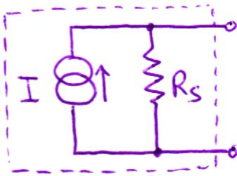
if  $R_s \gg R_L \Rightarrow$  close to an ideal current source
