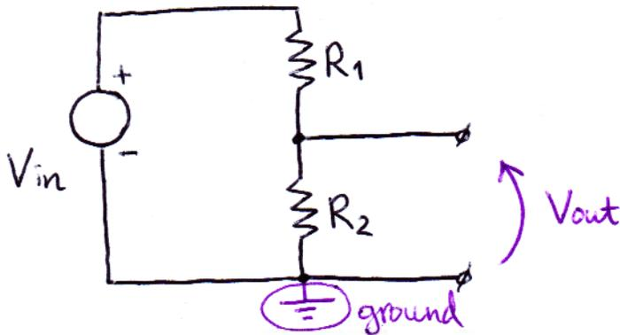
$$V_{out} = V_{in} \frac{R_2}{R_1 + R_2} \quad (\text{memorize})$$
