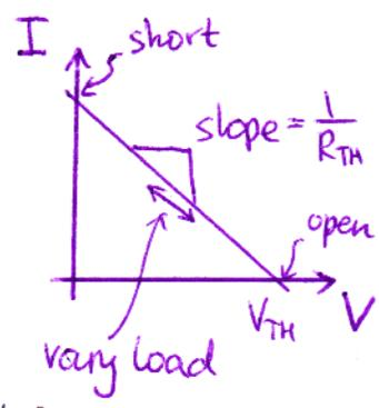
any combination of linear circuit elements with two output terminals may be replaced with ideal volt. source and series resistance
