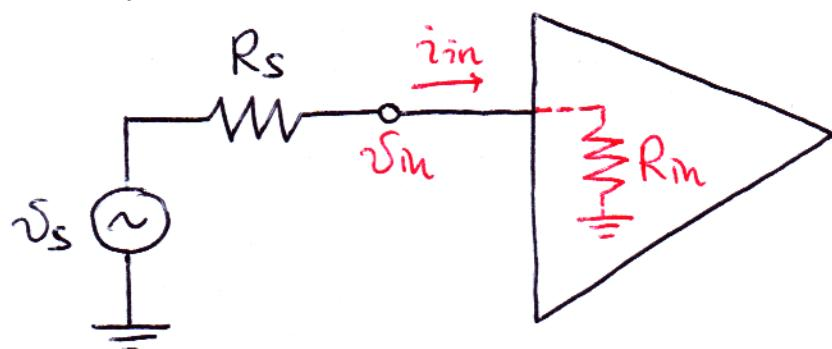
$$R_{\text{in}} = \frac{V_m}{i_{\text{in}}} (= \text{const})$$
