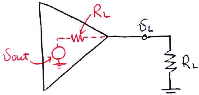
$$V_L = V_{out} \frac{R_L}{R_L + R_{out}}$$
