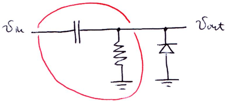
RC form HP filter: C blocks DC of  $v_{in}$  (e.g. scope's AC coupling mode)
