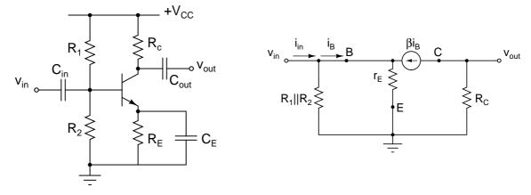
$v_{out} = -i_C R_C = -\beta i_B R_C$  and  $v_{in} = i_E r_E = (\beta + 1)i_B r_E$ . The resultant gain
