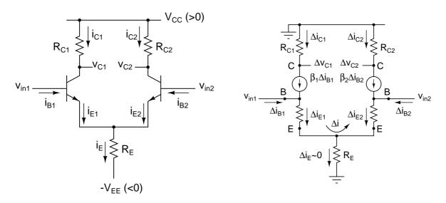
The power supply voltage  $V_{EE}$  is chosen to be large enough so that the emitter voltages fluctuations due to  $v_{in1}$  and  $v_{in2}$  do not change the current flowing through  $R_E$  resistor. That current, which is roughly  $(V_{EE} - 0.6V)/R_E$  assuming  $v_{in1}$  and  $v_{in2}$  are small signals, is to a very high degree independent of the input voltages.
