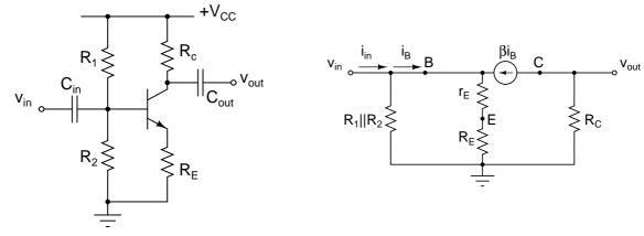
$v_{out} = -i_C R_C = -\beta i_B R_C$  and  $v_{in} = i_E (r_E + R_E) = (\beta + 1) i_B (r_E + R_E)$ . The resultant gain
