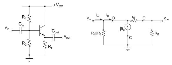
From the small-signal equivalent circuit we find that  $v_{out} = i_E R_E = i_B(\beta+1)R_E$ , and  $v_{in} = i_E(r_E+R_E) = i_B(\beta+1)(r_E+R_E)$ . Thus, the voltage gain is
