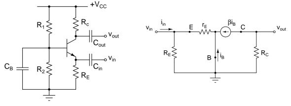
We write for the output  $v_{out} = -i_C R_C = -\beta i_B R_C$ . The input  $v_{in} = -i_E r_E = -(\beta + 1)i_B r_E$ . The resultant gain
