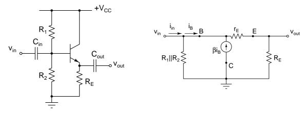
From the small-signal equivalent circuit we find that  $v_{out} = i_E R_E = i_B(\beta+1)R_E$ , and  $v_{in} = i_E(r_E+R_E) = i_B(\beta+1)(r_E+R_E)$ . Thus, the voltage gain is
