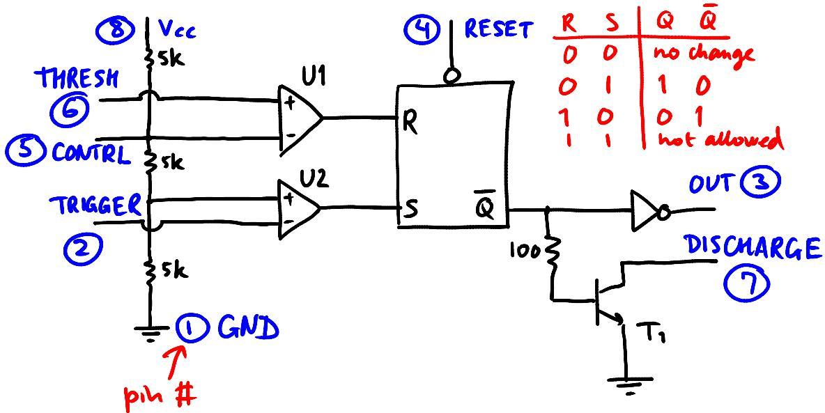
2 Comparators      RS latch      saturated switch
