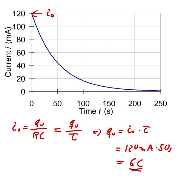
The graph shows the electric charge on a charging capacitor in a simple *RC* circuit.
