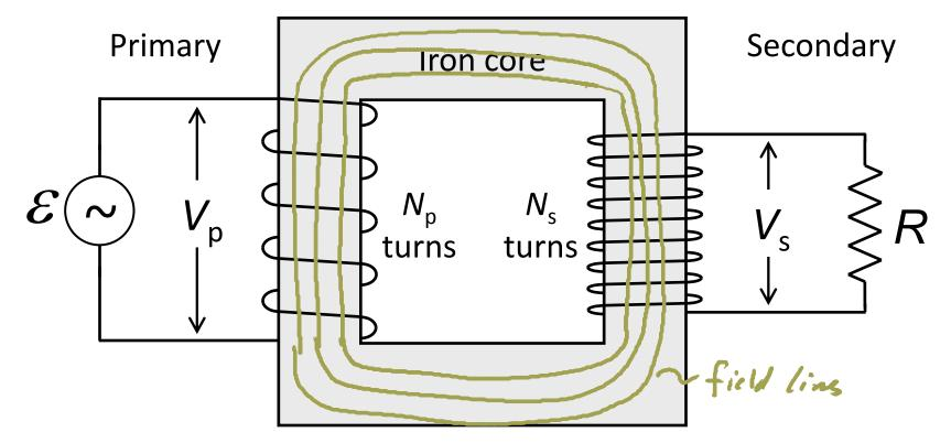
The iron core ensures that the  $\Phi_B$  per turn is the same in both the primary & secondary windings.
