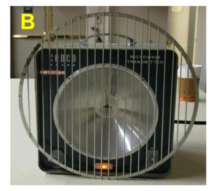
The electric dipole antenna of the microwave transmitter is vertical. Which orientation of the metal grill will allow the highest transmission of microwaves?
