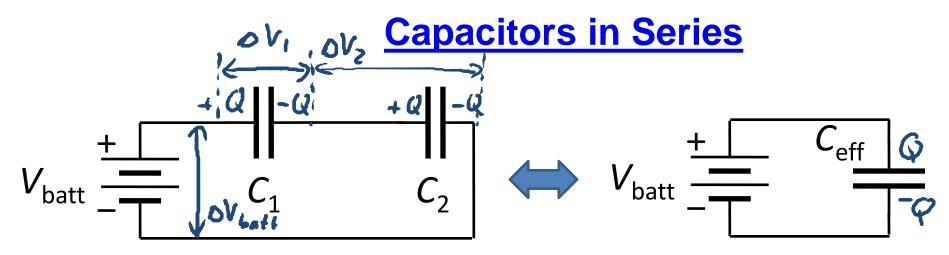
What should be the value of  $C_{\text{eff}}$  in terms of  $C_1$  &  $C_2$  so that the battery delivers the same charge in both circuits?
