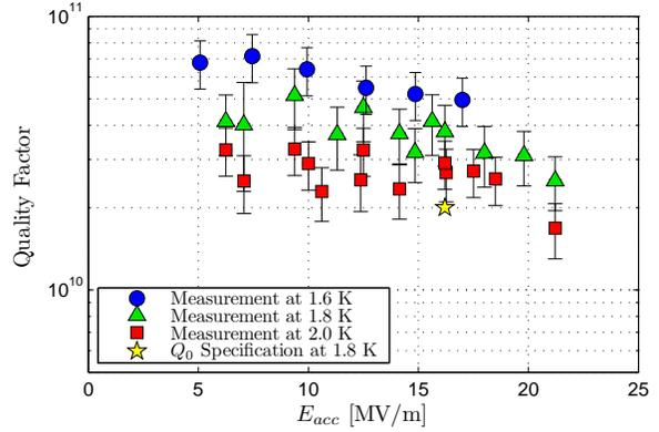
Figure 5: Initial  $Q_0$  vs E measurement of ERL 7.1 in HTC-3. The star denotes the design specification for 1.8 K operation. The cavity field reached 21.2 MV/m, limited by available pumping capacity. Radiation at highest fields was  $< 1$  R/hr. The large uncertainties in the 1.6 K points arises from the small level of dissipated power, but are consistent with BCS predictions for a very low residual resistance cavity.
