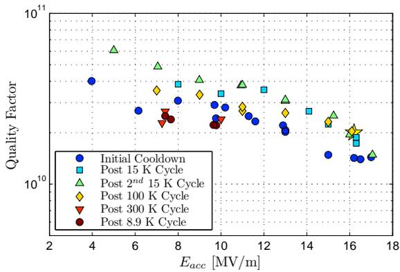
Figure 3:  $Q_0$  vs  $E_{acc}$  measurements at 1.8 K before and after thermally cycling the ERL 7-1 in the HTC-2 experiment. Star denotes 1.8 K  $Q_0$  specification. The most benefit in reduced surface resistance (higher  $Q_0$ ) was obtained after the first 15 K thermal cycle. For visual clarity, 20% error bars in  $Q_0$  have been suppressed.
