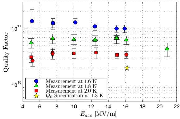
Figure 6: Final  $Q_0$  vs  $E_{acc}$  measurement of ERL 7.1 in HTC-3. At the operating accelerating gradient and temperature, the cavity's  $Q_0$  exceeds design specification by a factor of three, reaching  $6 \times 10^{10}$ . Accelerating gradients of 21 MV/m were achieved.
