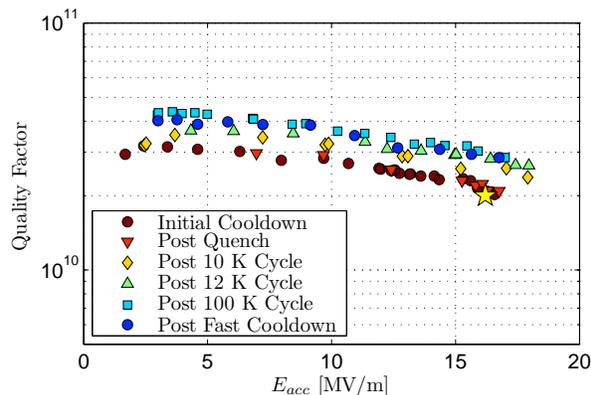
Figure 1:  $Q_0$  vs  $E_{acc}$  measurements at 1.8 K before and after thermally cycling ERL7-1 in HTC-1. The star denotes the  $Q_0$  specification at 1.8 K. The  $Q_0$  at design gradient increased by  $\sim 50\%$  after thermally cycling to low temperatures. 10% error bars in  $Q_0$  are suppressed for visual clarity.
