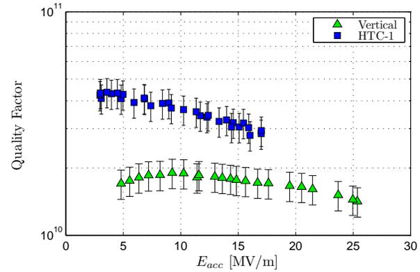
Figure 8: Comparison of  $Q_0$  vs E measurements of ERL 7.1 in the vertical test and HTC-1. Both data sets were taken at 1.8 K. HTC-1 exhibits much higher  $Q_0$  than in the vertical case, even though no surface processing was done between the two measurements.
