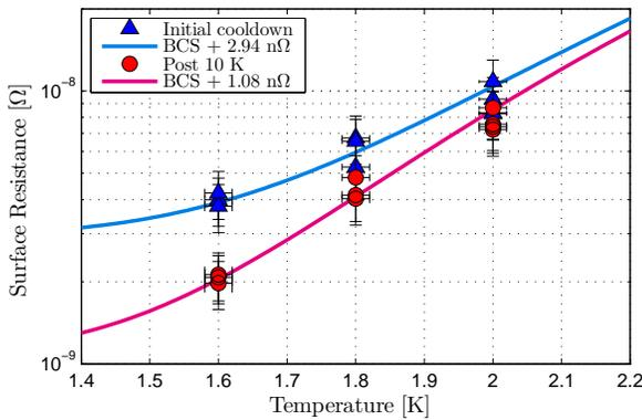
Figure 7:  $R_s$  vs temperature measurements before and after thermally cycling ERL 7.1 to 10 K in HTC-3.
