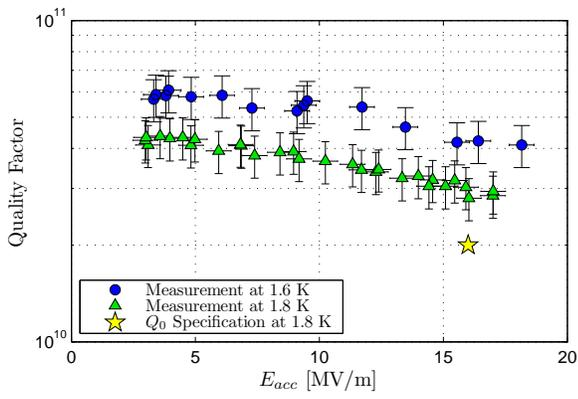
Figure 2: Final  $Q_0$  vs  $E_{acc}$  measurement of ERL 7.1 in HTC-1.
