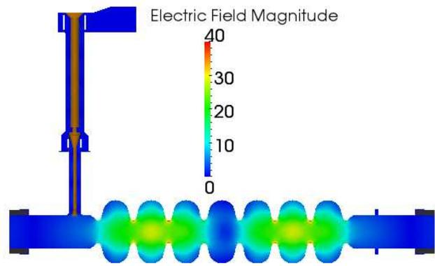
Figure 1: Magnitude of the electric field (in arbitrary units) for a dipole mode in the lowest HOM passband. The absorbing load is in gray, and the white areas are alumina dielectrics isolating the cavity vacuum space from the cold and warm spaces.
