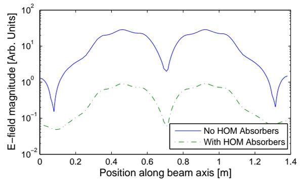
Figure 2: Simulated magnitude of electric field component along a line parallel to the beam axis and offset toward the high power coupler by 1 mm for a geometry with and without absorbing loads. The absorbing load properties were  $\epsilon = (50 - 25i)\epsilon_0$  and  $\mu = \mu_0$ . The presence of the HOM load significantly reduces the electric field amplitude near the beam axis.
