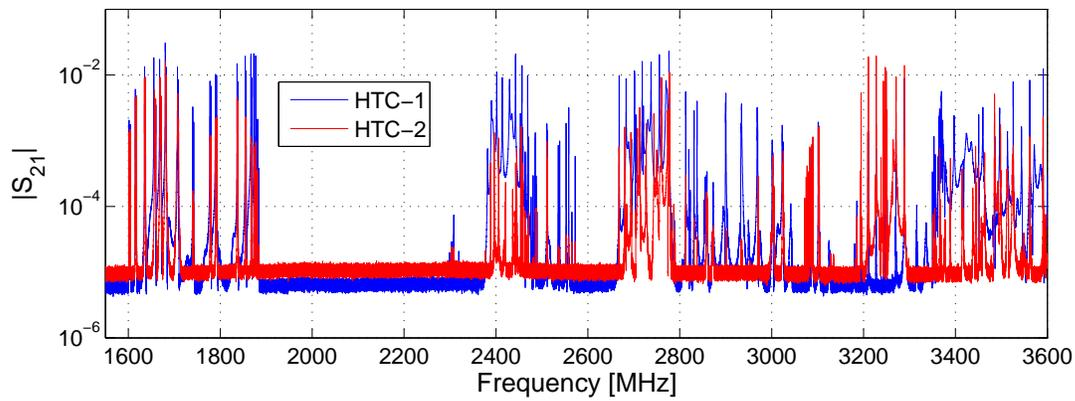
Figure 3: Amplitude of the scattering parameter  $S_{21}$  in the first two HTC experiments. The large quality factor of the modes are due to the fact that there were no HOM loads installed in HTC-1 and HTC-2. The mode frequencies agree with 2D simulations.
