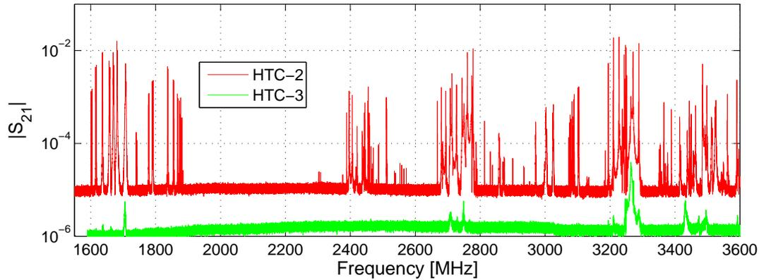
Figure 4: Amplitude of the scattering parameter  $S_{21}$  in the HTC-2 and HTC-3 experiments. The only significant change between the two runs is the beamline HOMs in HTC-3, showing strong damping of all modes.
