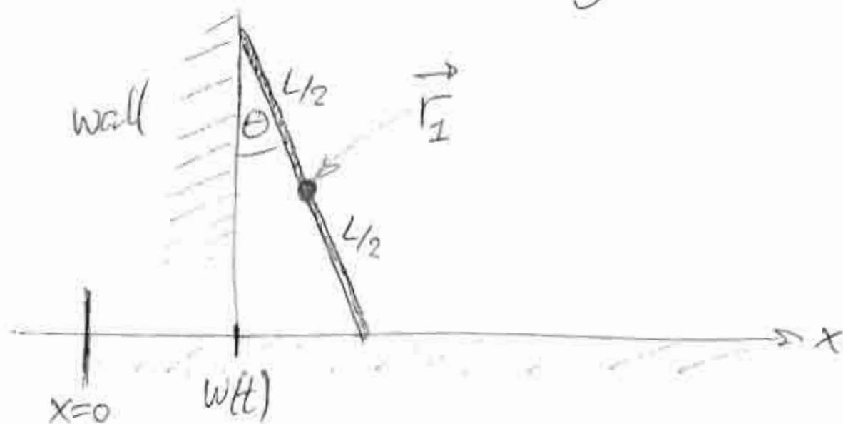
$$\begin{aligned}\vec{r}_1 &= \text{position of ladder CoM} \\ &= x\hat{x} + y\hat{y}\end{aligned}$$
