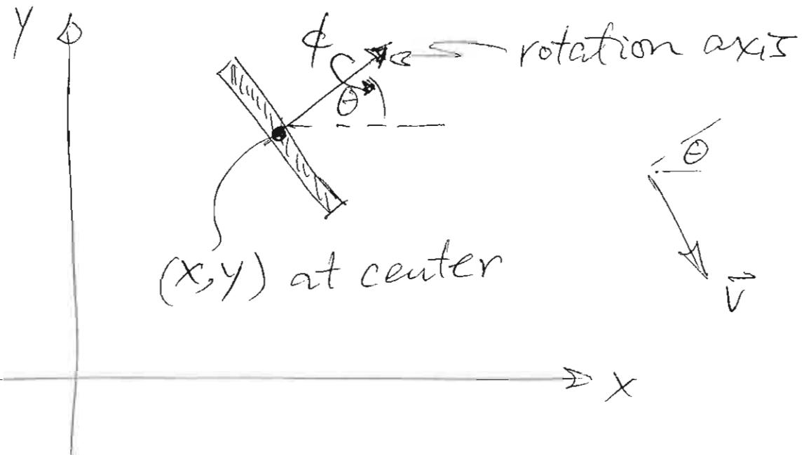
$$(\text{velocity of center}) = (\text{velocity of contact point}) = r\dot{\phi} \\ = v$$
