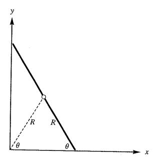
The center of mass of the ladder is halfway between the ends and is also indicated in the drawing to help you in your calculations. Use the tilt of the ladder,  $\theta$ , as the generalized coordinate for this one-degree-of-freedom system.
