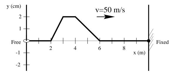
A stretched cable of mass density  $\mu=4$  kg/m has a free boundary condition at x=0 and a fixed boundary condition at x=10m. An asymmetric pulse is traveling in the +x direction at a velocity v=50 m/s. At t=3 seconds the pulse is 2cm high, and shaped as shown in the graph above.
