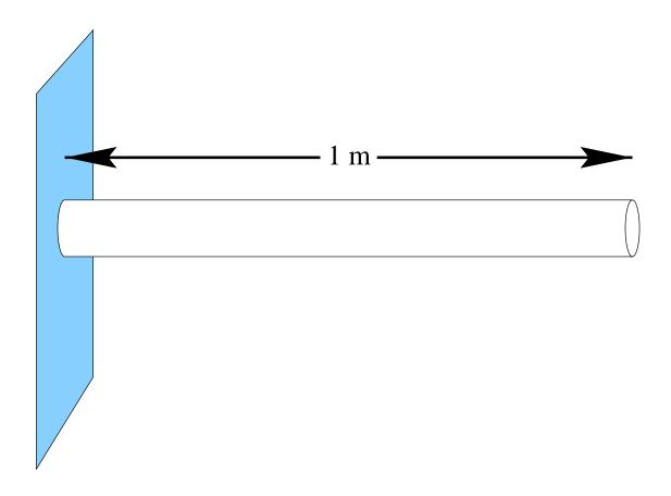
A one meter aluminum rod is hanging horizontally in the air. On the left at x=0, it is rigidly clamped at the wall (no longitudinal motion possible at x=0). On the right at x=1 m, it is hanging freely in the air (as were both ends of the rod in Experimental Lab I).
