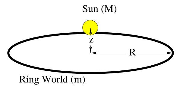
If the ring is displaced a distance z perpendicular to the plane of the ring, one can use Newton's universal law of gravitation to write the force on the ring in terms of the gravitational constant G. For small z and  $m \ll M$ , the ring accelerates according to the equation
