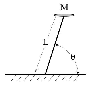
In this problem, we will explore the behavior of the pole and plate, treating it as a simple, undamped pendulum, for angles near the *unstable* equilibrium. We remind you that the equation of motion for the angle of the pole with respect to the ground (*not* the angle with respect to the vertical!) is
